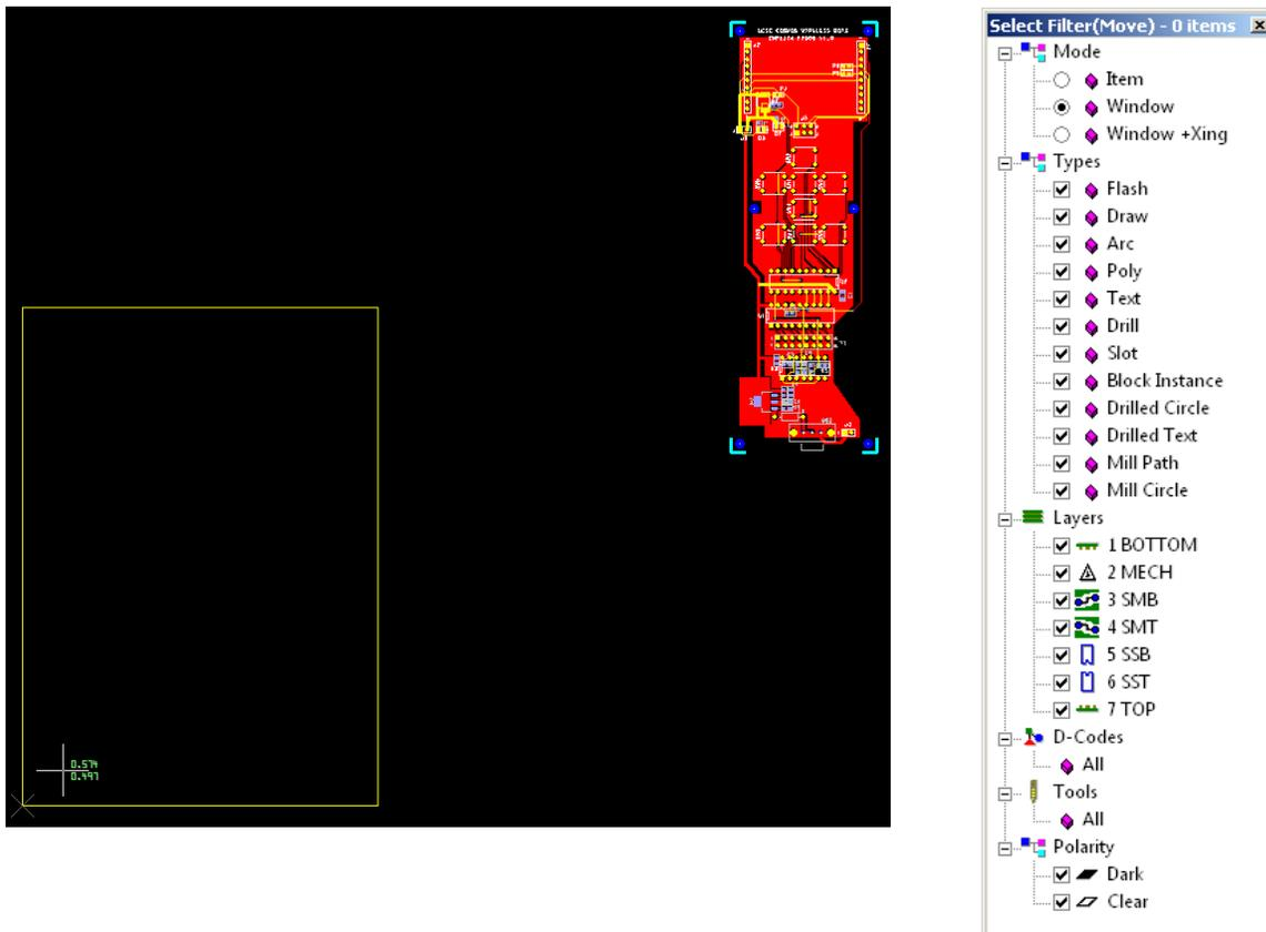
If the Units and Precision were correctly set to “Inches” and “1/1000...” earlier (see page 5), then the cursor cross-hair should be showing three decimal points. Moreover, the pcb layout is probably outside the 5.000 X 7.000 inch film box as shown in the screen shot. The objective is to select everything on all 7 layers and move them so the lower-left cut mark is precisely aligned with the film box’s lower left reference corner at the coordinate origin.
